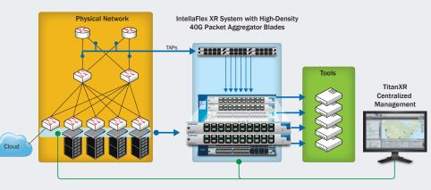
The high-density 40G blade can aggregate, filter, and load balance traffic into IntellaFlex XR systems for advanced processing before sending traffic on to connected tools.
